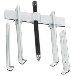
NOTE: Puller removes a gear with two sets of straight jaws, bolted together for extra reach. Set comes with two sets of jaws — Jaw No. J4015 has a 4-11/16" reach and No. J4016A has a 7-1/8" reach. Bolted together they easily clear the 8" long gear shaft.
